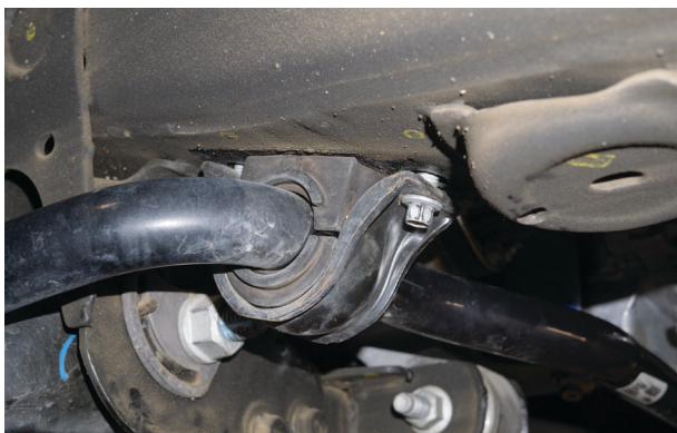
Fig. 2: Loosen the sway bar brackets.
