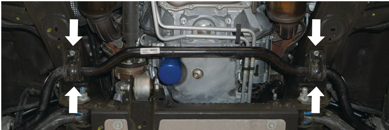
Fig. 1: Loosen the sway bar brackets.
